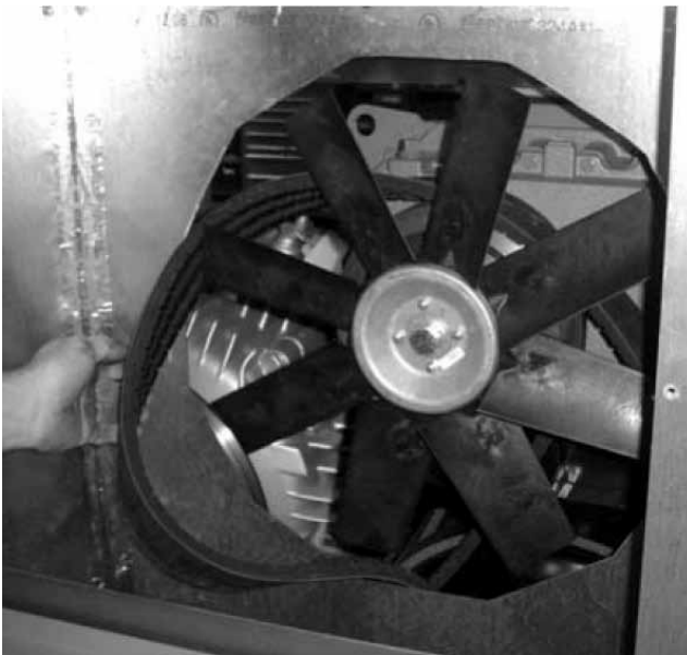
(6) Pull the belt out through the clearance between the fan OD and the panel hole.
