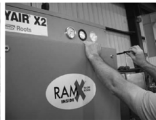
(5) HOLD THE DOOR, PUSH AND TURN THE KEY ¼ TURN CLOCKWISE AND REMOVE THE KEY. LIFT UP AND REMOVE THE RIGHT SIDE DOOR PANEL.
