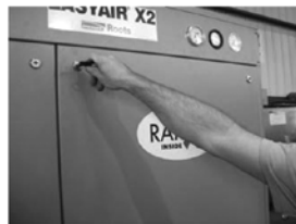
(1) INSERT THE KEY IN THE LEFT KEY HOLE OF THE DOOR PANEL.
