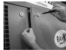
(3) HOLD THE DOOR OPEN, PUSH AND TURN THE KEY ¼ TURN COUNTER CLOCKWISE AND REMOVE THE KEY.
