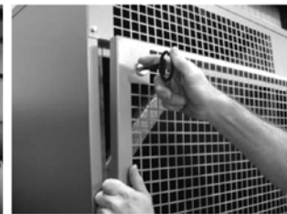
(6) FOR REMOVAL OF THE LEFT DOOR PANEL, USE THE PROCEDURE PER (2 & 3) ABOVE TO UNLOCK THE LEFT LATCH, AND (4 & 5) TO UNLOCK THE RIGHT LATCH.
