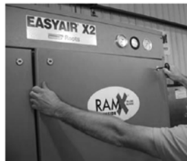
(4) HOLD THE DOOR OPEN WITH LEFT HAND, INSERT KEY IN THE RIGH HOLE, PUSH AND TURN THE KEY ¼ TURN COUNTER CLOCKWISE, PULL THE DOOR OPEN.
