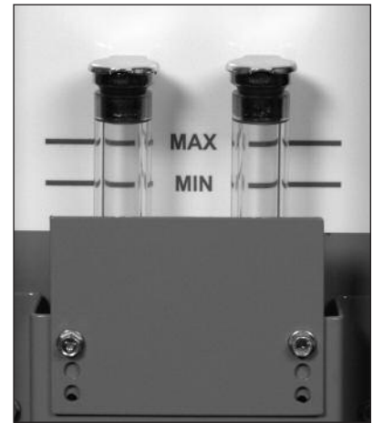
Oil fill level site glass.
